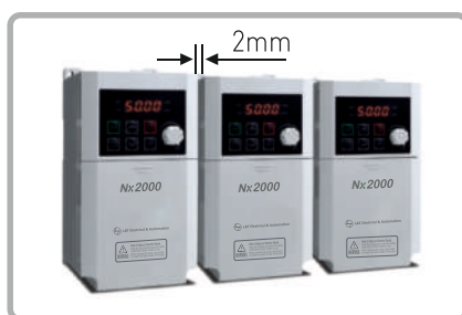
Side-by-Side Installation (2mm between drives)
