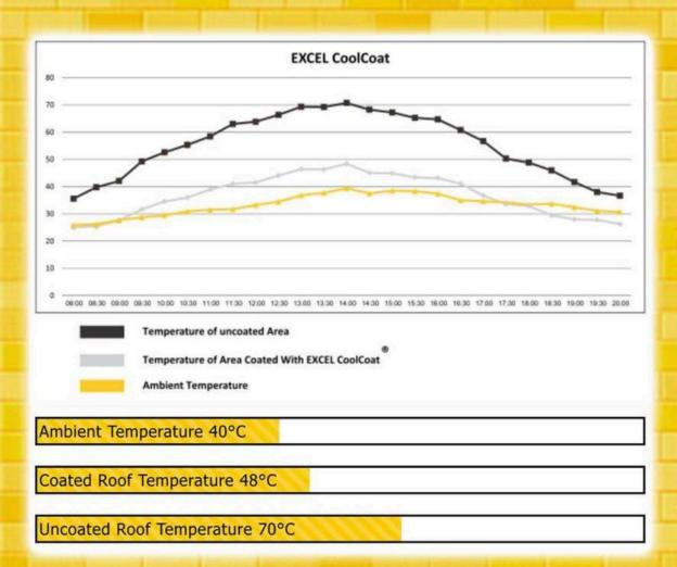
Temperature difference of around 22 °C note between the coated and uncoated surface.
