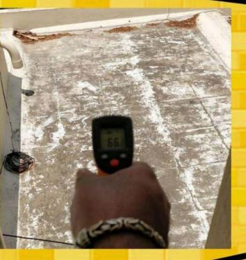
Temperature of Uncoated Roof 66° C
